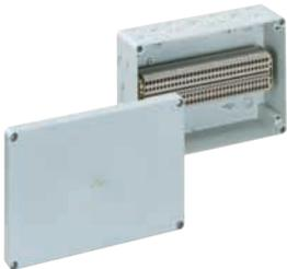
Terminal block enclosure, with standard rails NS 35, incl. 8 attachment bushes M20, seal range 8 - 13.5 mm, IP54, 2 attachment bushes M25, seal range 9 - 18.5 mm, IP54, 1 attachment bush M32, seal range 13 - 23 mm, IP54
