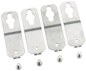
External fixing lugs, for mounting separate enclosures or small units on flat wall surfaces, can be fixed to the box base at an angle of 0°, 45°, or 90°, wall gap 7 mm, material stainless steel, suitable for all AK enclosures from 300 mm front,
