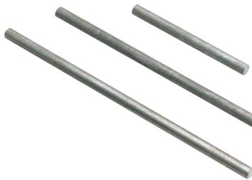
Support spars for various wall thicknesses in opposing formwork, always used in conjunction with blank base or back mounted box, spar length = wall thickness minus 1 cm, 2 support spars per socket, 4 support spars for extreme loads
