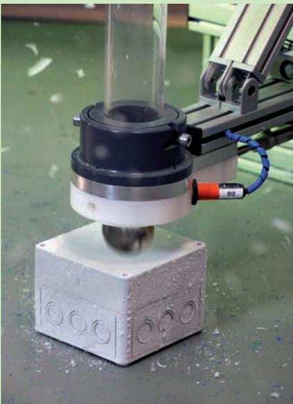
The splinters are ice residue from the cooling process at  $-35^{\circ}\text{C}$ .
