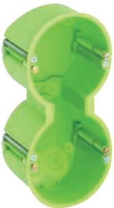
Cavity wall double socket, flame resistant, for plate thicknesses from 1 to 40 mm, with moulded patented combi jumpers and punching tool, device screw spacing 60 mm
