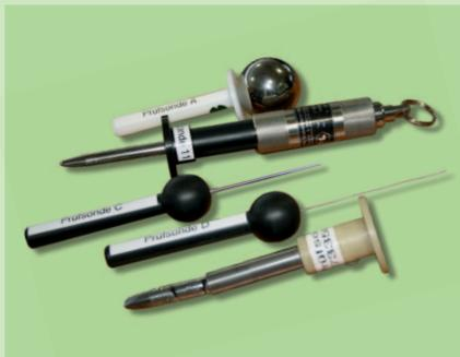
Test probe according to DIN 60529
