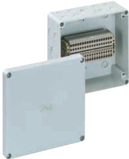
Terminal block enclosure, Polystyrene, grey, similar to RAL 7035, incl. 8 attachment bushes M20, seal range 8 - 13.5 mm, IP54, 2 attachment bushes M25, seal range 9 - 18.5 mm, IP54, 1 attachment bush M32, seal range 13 - 23 mm, IP54
