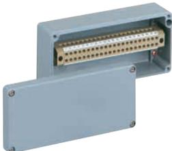
Terminal block enclosure in compact design - Industrial Quality - Aluminium, powder-coated painting silver grey RAL 7001, equipped with 22-pole terminal block 0.2-4 mm<sup>2</sup> (screw connection)
