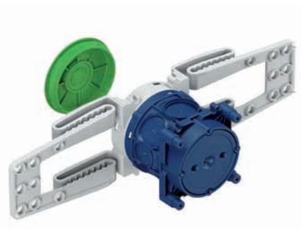
Reinforcement box, in two parts, green rearward base with max. 1 x 25 mm insert, combinable, Suitable for opposing formwork without support, pre-installation in the reinforcement bars, for concrete installation, combination possibility with the standard spacing 71 mm
