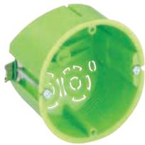
Cavity wall lighting connection socket, flame resistant, for plate thicknesses from 0.5 to 33 mm, with M5 brass bush to take a ceiling hook from the accessory range, acc. to DIN EN 60670-21, but max. loading on hook 20 N (2 kg)
