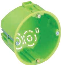
Cavity wall receptacle, flame resistant, universal socket for plate thicknesses from 1 to 40 mm with moulded patented combi jumpers and punching tool, device screw spacing 60 mm
