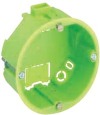
Cavity wall flat box, flame resistant, special box with small installation depth (35 mm), for thin walls with plate thicknesses from 1 to 20 mm, with moulded patented combi jumpers, device screw spacing 60 mm
