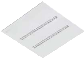
PANEL INDIVILED 625 DALI UGR<19 GEN 2 Square recessed panel luminaires with Multi Select, DALI-2 IoT driver, EVERLOOP design and low glare, 625 x 625 mm
