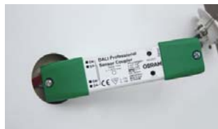
02 Pass the sensor coupler through the ceiling aperture
